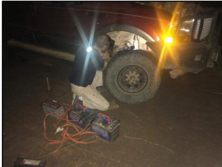
Welding the frame with batteries
